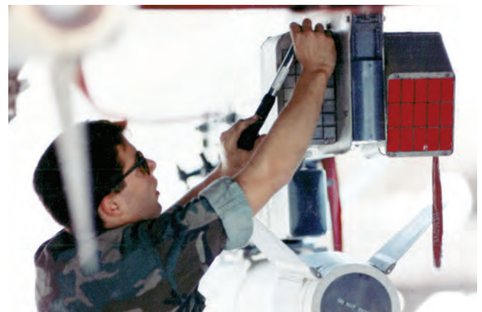
A weapons specialist loads chaff and flares aboard an F-4G. The missile is an AGM-88 HARM. [USAF]
